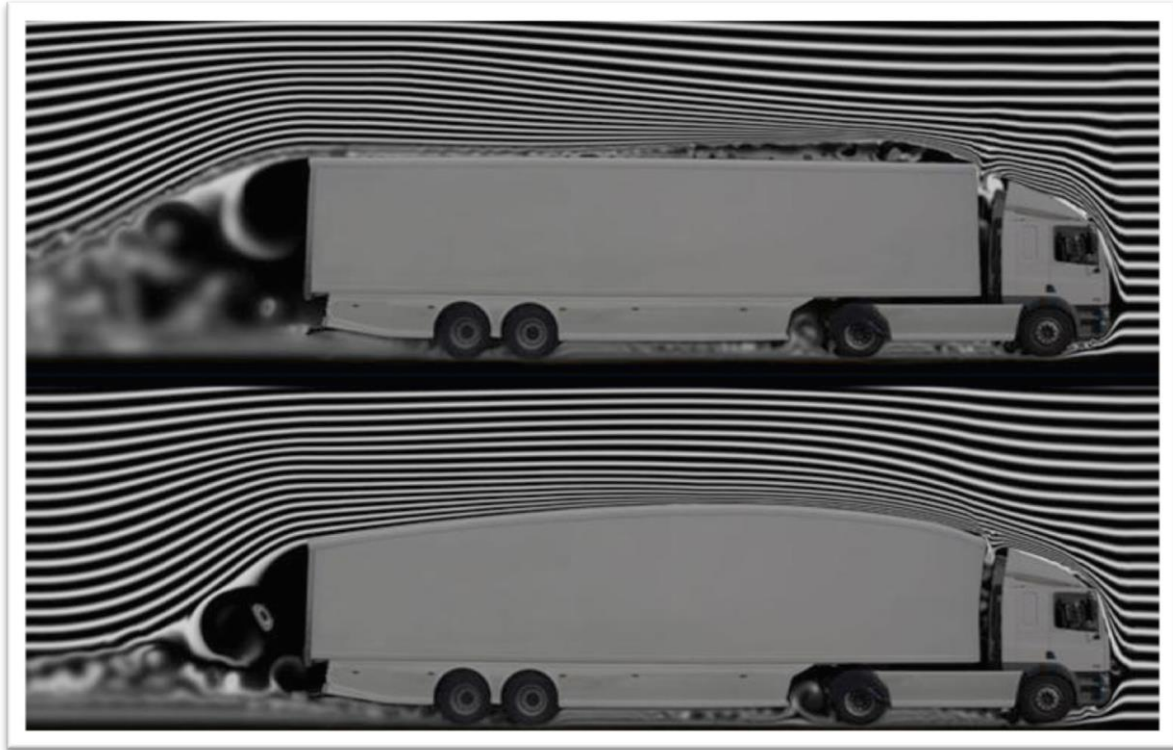
Fig 1. Comparison of aerodynamic performance between a conventional cab and trailer (top) and a teardrop design
